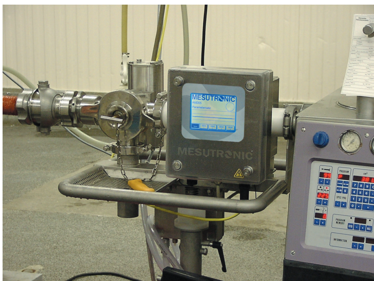
Metal Separator P-TRON 05 O TOUCH installed on a Vacuum Filler
